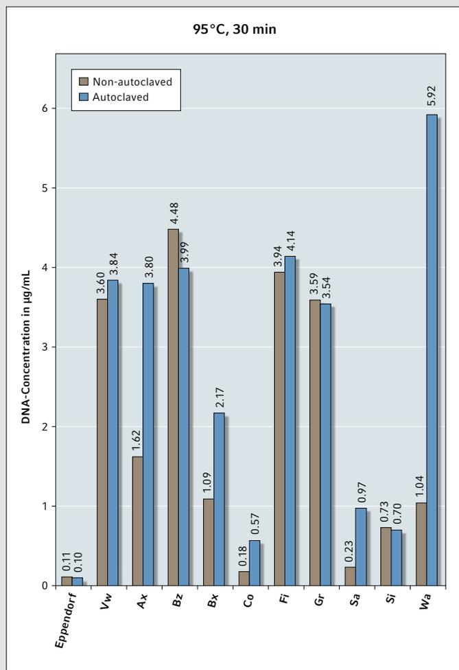
**Fig. 2:** False DNA concentration ( $\mu\text{g/mL}$ ) based on UV-absorbing leachables, which had been released from micro test tubes into ultra-pure water samples after incubation at  $95^\circ\text{C}$ , 30 min. Mean values of 24 pooled samples from non-autoclaved (brown bars) and autoclaved (blue bars) tubes are shown.
